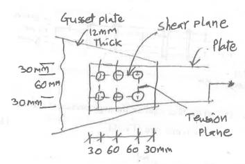
(c) Design a bridge diagonal subjected to a factored tensile load of 300 kN. The length of the diagonal is 3.0 m. The tension member is connected to a gusset plate 16 mm thick with one line of 20 mm diameter bolt of grade 8.8.
